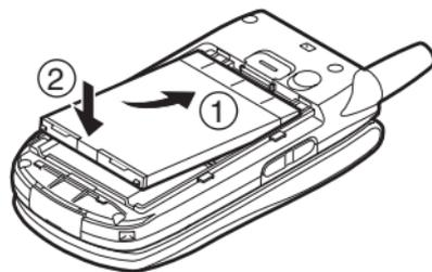
4. Replace the battery cover and slide it as shown below.
