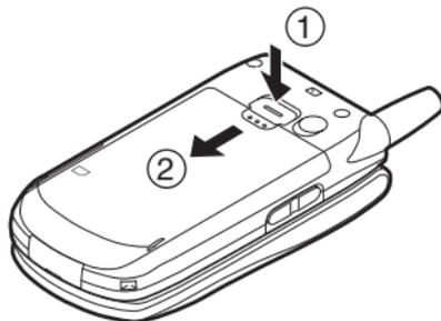
2. Pick up the battery using the protruding edge and remove the battery from the phone.
