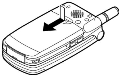
2. Pick up the battery using the protruding edge and remove the battery from the phone.
