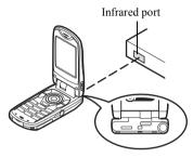
Infrared ports need to be placed within 20 cm of each other and within a 30° angle.
