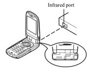
• Infrared ports need to be placed within 20 cm of each other and within a 30° angle.
