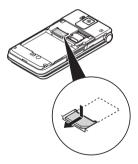
4. Hold the battery so that the metal contacts are facing down and slide them into the slots. Close the cover.
